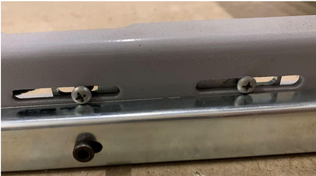
Tighten the screws to adjust the position of the sensor.
