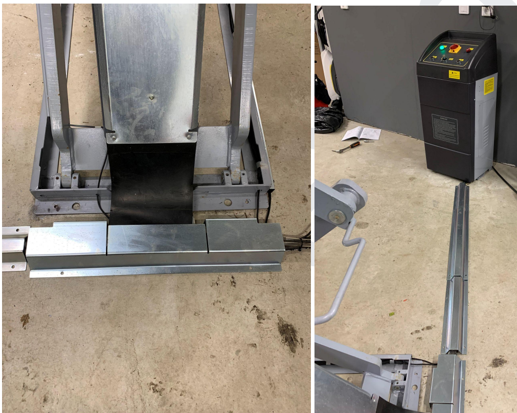
Cover plate at platform (picture on the left) and cover plate for control box (picture on the right)
