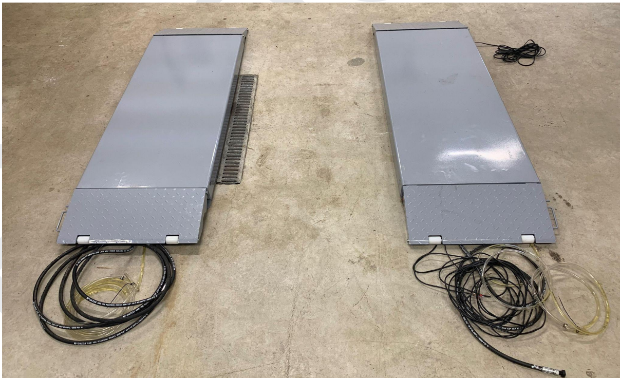
The sub-platform with hoses (left) & the main platform with hoses & sensor cables. (to the right)
