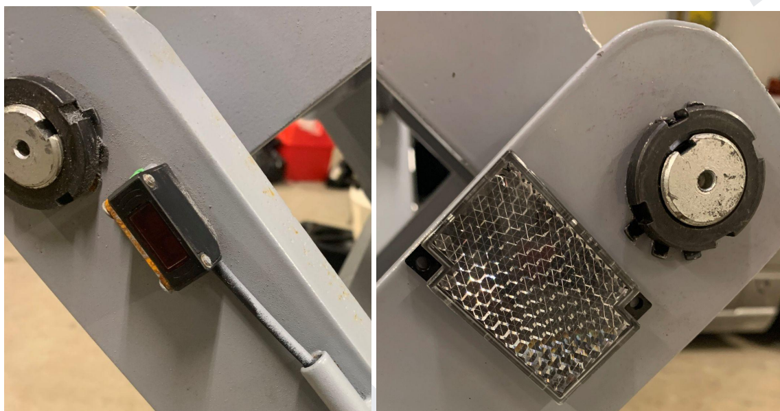
The photoelectric safety stop sends a signal via reflex to the control box.
