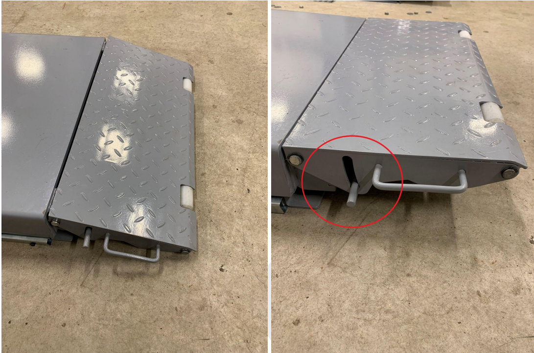
Ramp in lowered position (picture to the left) & raised position with the latch circled. (picture to the right)
